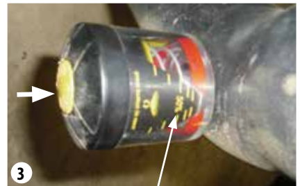
Air filter clogging indicator
