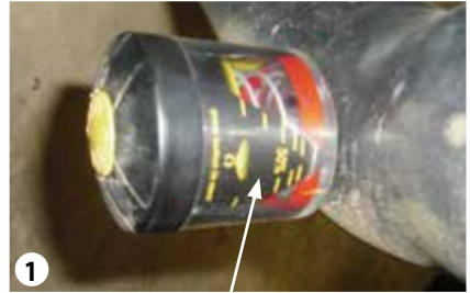
Air filter clogging indicator
