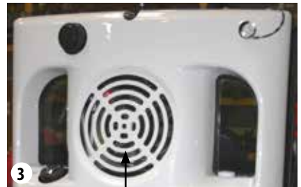
Air conditioning condenser
