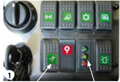
1 High-pressure cleaner switch Water level gauge
